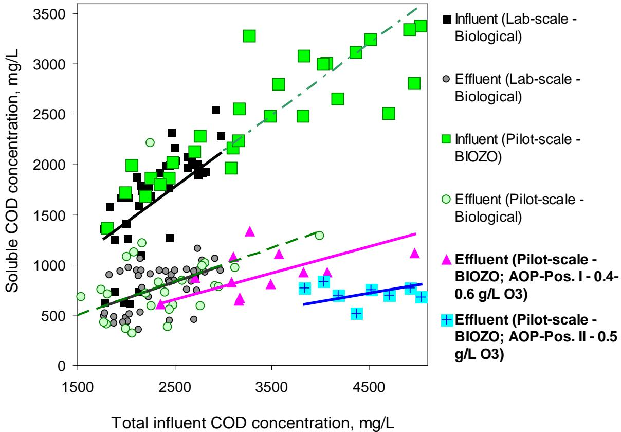
Combined operation with AOP installed upstream to the aerobic zone is an effective means to decrease COD<sub>Soluble,Eff</sub>, thereby keeping it below 1000 mg/L COD.
