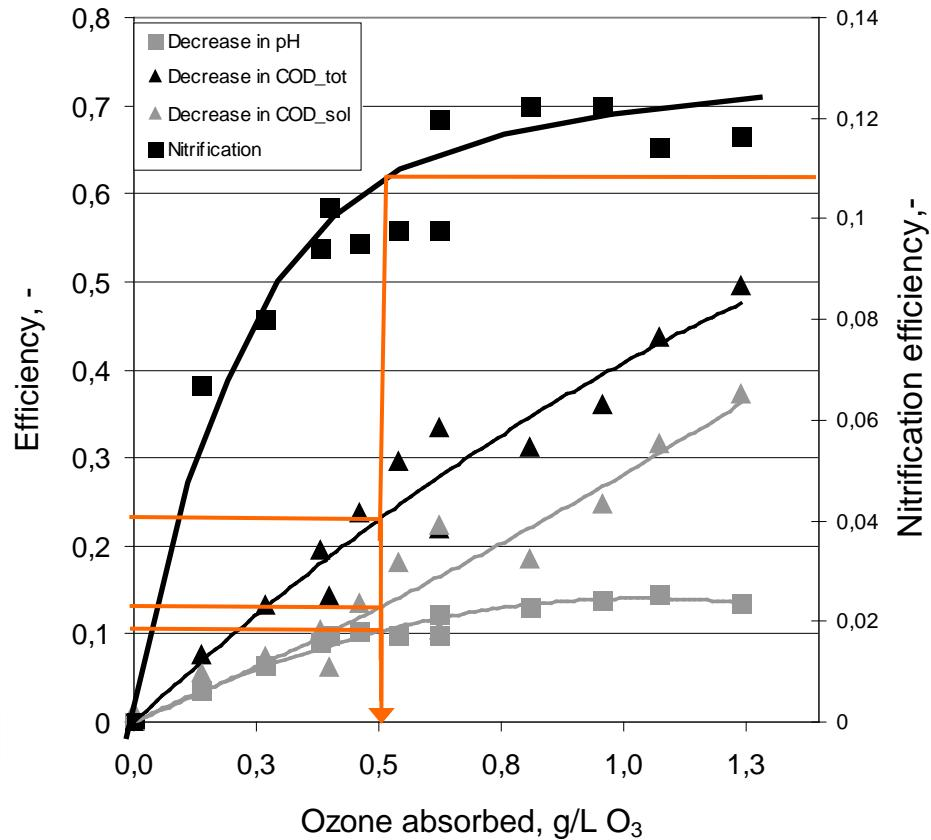
**Using the effluent of the biological treatment system, an optimum ozone dosage of approx. 0.5 g/L  $\text{O}_3$  can efficiently :**
