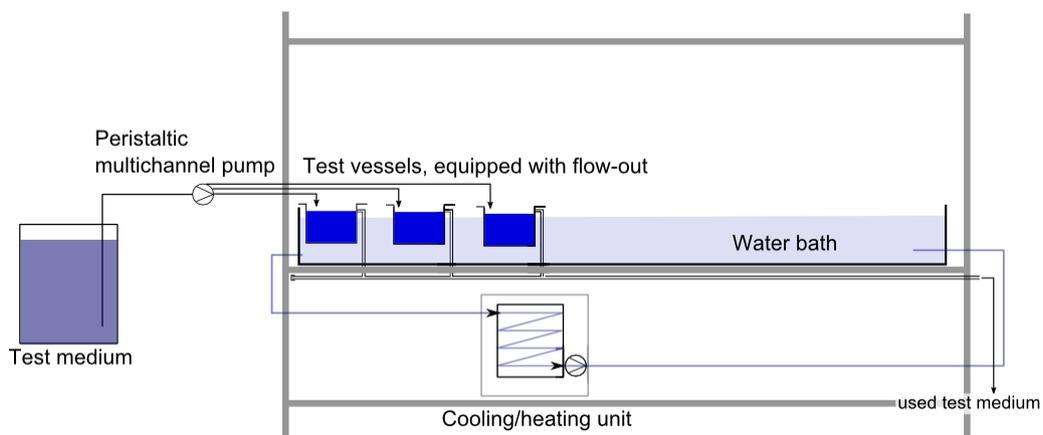
**Figure 1: Exemplary set up for a flow-through test with one test medium. Temperature of the test medium is controlled indirectly via a regulated water bath.**
