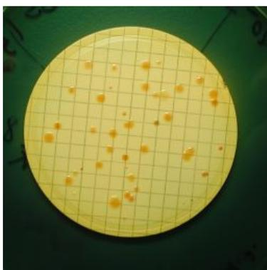
**Figure 3.2 Membrane filter with coliform bacteria on TCC-agar**
