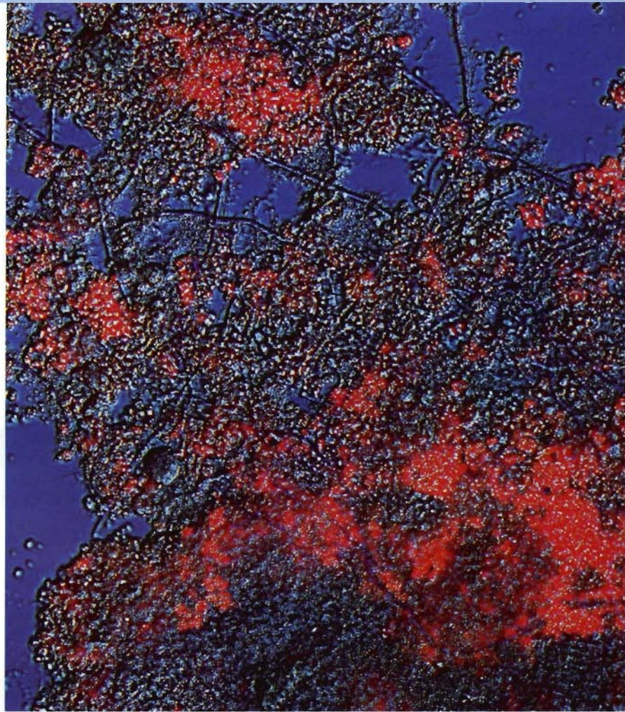
Micrograph of fluorescently stained (Nile Red) activated sludge treating industrial wastewater enriched for PHA production. Floc structure is shown at 200x with interference contrast. Red zones suggest regions of activity in biopolymer storage. Image courtesy Petter Lind
