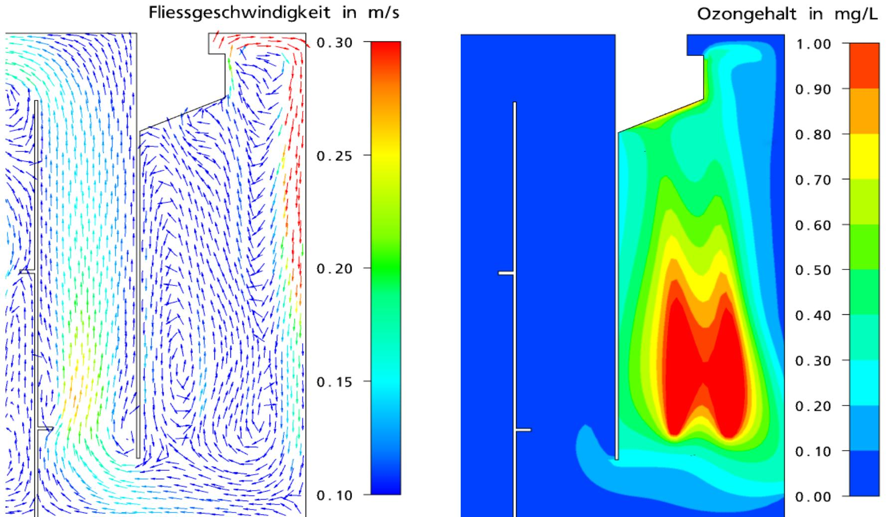
Three-dimensional CFD-simulation for  $Q = 0.15 \text{ m}^3 \text{ sec}^{-1}$ , and  $\text{O}_3\text{-dosage} = 5 \text{ g m}^{-3}$
